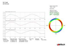
The developed views provide the possibility to evaluate the part at any diameter.
